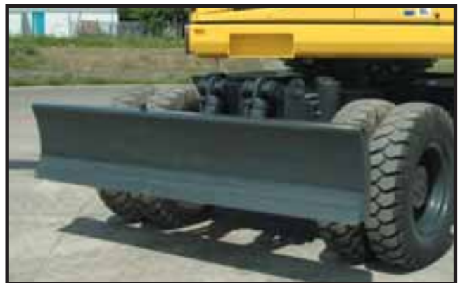
Dozer blade A parallel blade is available with standard cylinders protector for both the front and rear of the machine.
