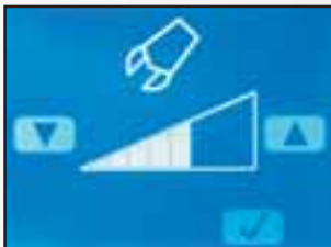
Fine tune hydraulic flow adjustment screen in A (active) or E (economy) mode
