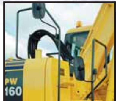
Large handrail for safe access
