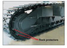
**Sturdy guards** shield the travel motors and piping against damage from rocks.
