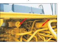
Metal Guard Rings Metal guard rings protect all the hydraulic cylinders and improve reliability.
